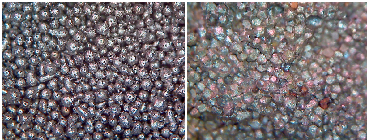
Pic. 16: Stellite granules on steel; left before, right after explosion
