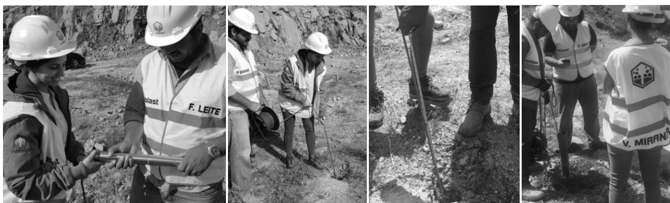
Figure 7. Field Procedure from left to right: probe assembling; probe deployment; offset measurement; measurement time record
