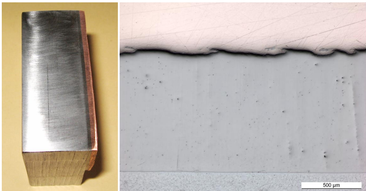
Pic. 15: Triple layer; below steel; mid titanium; on top copper
