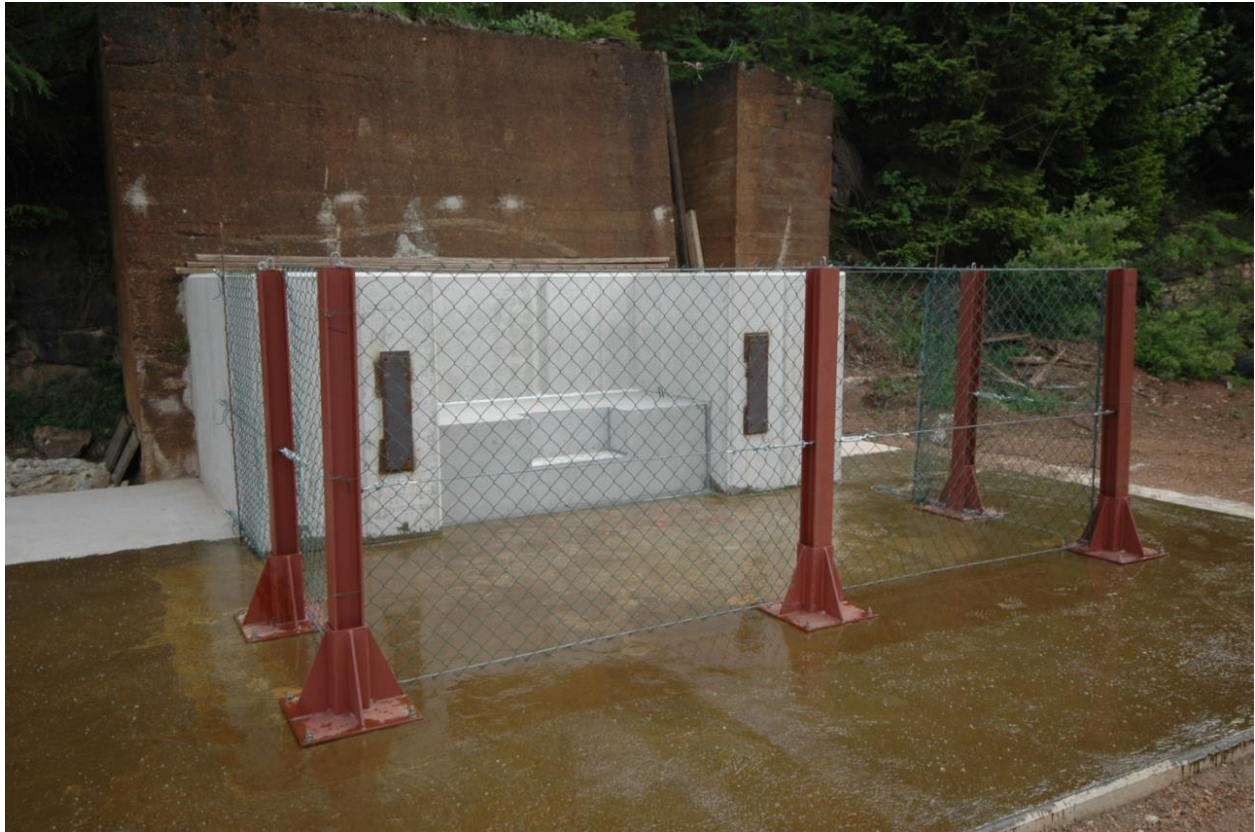
Figure 1 –Yokes at the Erzberg blasting site. They allow waves to escape from a test specimen. The inner yoke has room for the block.
