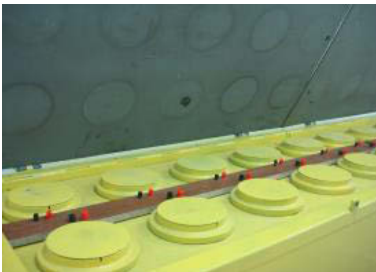
Fig.2. Stand for testing electric detonators as required by harmonized European standards
