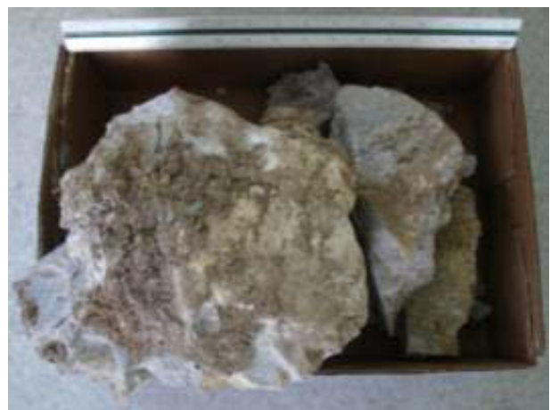
Example 1: Secondary school in the vicinity of a quarry with blocks landing in the playground approximately 300 m in front of the blast
