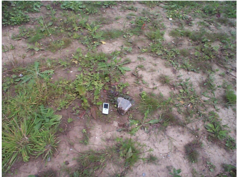
Example 6: Blocks landing in a field and another impact on a dwelling more than 430 m from the blast
