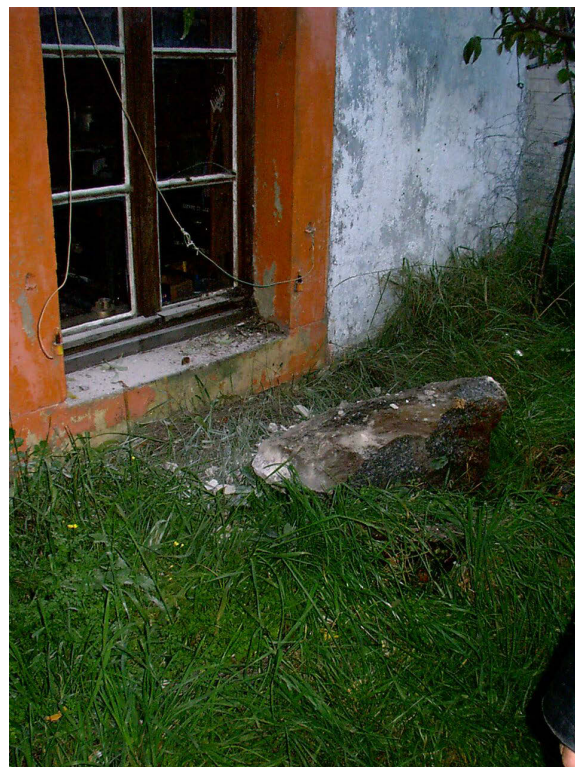
Example 5: Houses bordering a site road and blocks projected onto the frontage approximately 200 m from the blast
