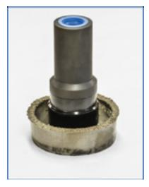
Tubular cutter for dril pipe.
